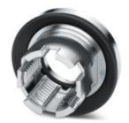
M12 threaded sleeve with tolerance-compensating function, for straight, SMD-solderable M12 socket contact inserts. Suitable for 1.6 mm  $\dots$  2.3 mm thick front plates.
