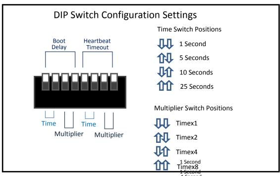
As an example, if the intention is to set a boot delay of 100 seconds, switches 1-2 would both be set in the up position for a time of 25 seconds, and switches 3-4 would be set of 4. This setting provides 25 seconds x4 for 100 seconds boot delay.
