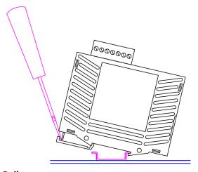
Removing from DIN-Rail
