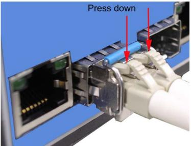
Figure 2.11: Remove LC connector
