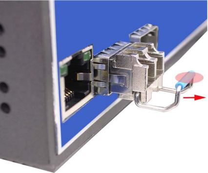
Figure 2.12: Pull out from the transceiver
