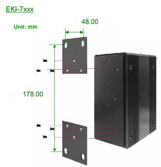
Figure 2.5: Combine the Metal Mounting Kit
