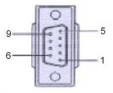
DB 9-pin Female Figure A.4: DB 9-pin female connector
