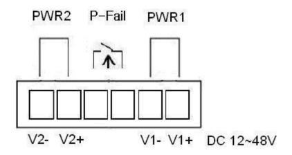
Figure 2.13: Pin Assignments of the Power Connector
