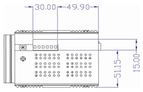
Figure 2.4: Top View of EKI-7659C
