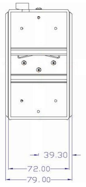
Figure 2.3: Rear View of EKI-7659C
