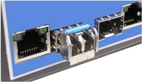
Figure 2.9: Transceiver Inserted
