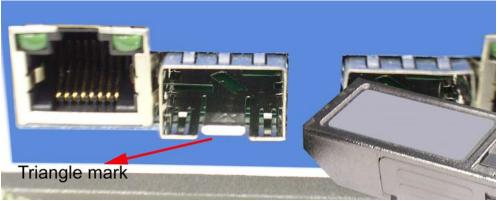
Figure 2.8: Transceiver to the SFP slot
