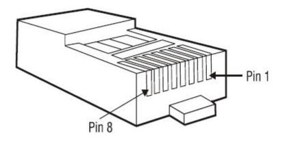
Figure A.1: RJ-45 Pin Assignments
