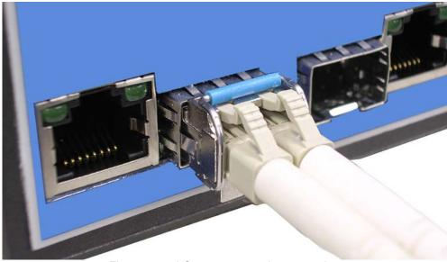
Figure 2.10: LC connector to the transceiver
