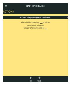
Trigger an action when a button is pressed, then trigger the same action again when the button is released.
