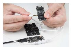
Now, plug the servo connector onto the Motion Board.
