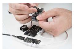
Finally, plug the Micro B end of the power adapter into the Director board, and the other end into the wall. You should see one solid light and one blinking light on the Motion Board and the Button board. On the Director Board, you'll see one solid light and one light which blinks one time, then pauses, then repeats. This shows that power is present and the boards are up and running.
