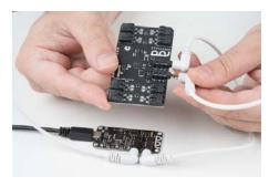
Plug the other end of that cable into the "In" jack on your Motion Board.
