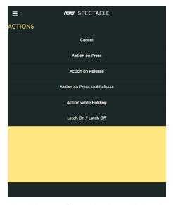
For the Button board, there are five options: three which produce a momentary pulse type output and two that produce a continuous switch type output.
