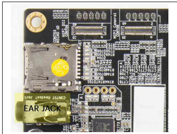
Figure 15. Ear Jack Interface location on the Platform Board
