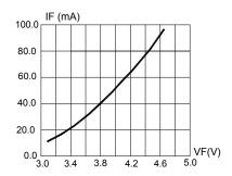
FIG.1 FORWARD CURRENT VS. FORWARD VOLTAGE.
