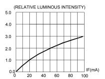
FIG.2 RELATIVE LUMINOUS INTENSITY VS. FORWARD CURRENT
