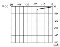
FIG.3 REVERSE CURRENT VS. REVERSE VOLTAGE.
