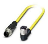
Sensor/Actuator cable, 3-position, TPE, yellow RAL 1021, Plug straight M12 SPEEDCON, A-coded, on Socket angled M12 SPEEDCON, A-coded, Cable length: 3 m
