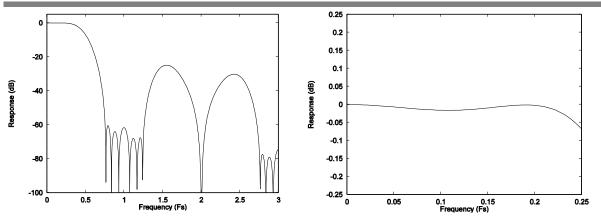
Figure 27 DAC Digital Filter Frequency Response – Type 3 Figure 28 DAC Digital Filter Ripple – Type 3
