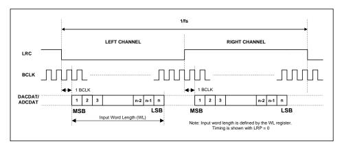
Figure 13 I<sup>2</sup>S Justified Audio Interface (assuming n-bit word length)
