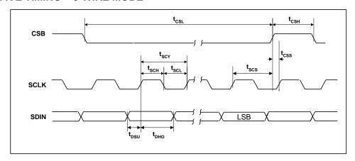
Figure 4 Control Interface Timing – 3-Wire Serial Control Mode
