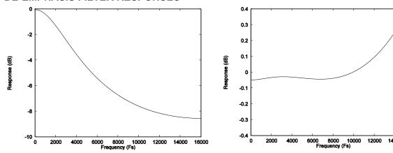
Figure 37 De-emphasis Frequency Response (32kHz)
