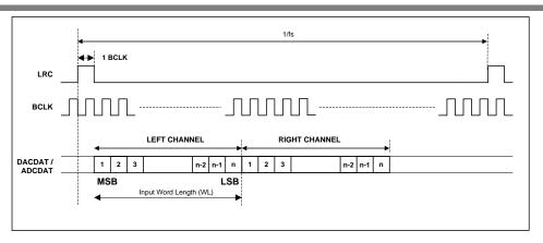
Figure 14 DSP/PCM Mode Audio Interface (mode A, LRP=0, Master)
