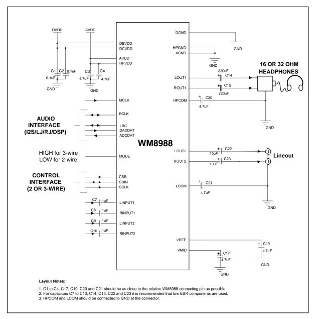
Figure 44 Recommended External Components Diagram
