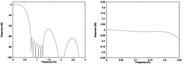
Figure 33 ADC Digital Filter Frequency Response - Type 2 Figure 34 ADC Digital Filter Ripple - Type 2
