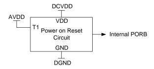
Figure 6 Internal Power on Reset Circuit Schematic
