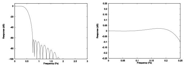
Figure 35 ADC Digital Filter Frequency Response – Type 2 Figure 36 ADC Digital Filter Ripple – Type 3
