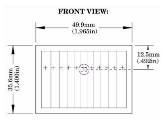
Figure 9. Flat Lens: AA 0.9 GI T1
