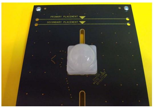
Figure 4. Assembled Clip-In Lens Installed on the ZMOTION 20-Pin Development
