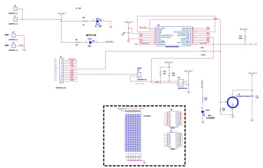
Figure 17. ZMOTION 20-Pin Development Board Schematic Diagram, #1 of 2
