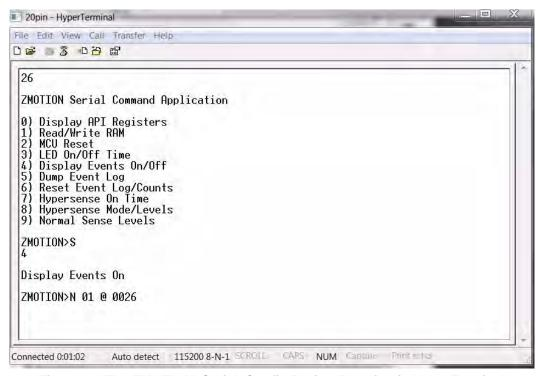
Figure 16. The ZMOTION\_Serial\_Config Project Running in HyperTerminal
