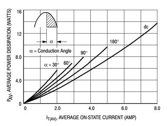
Figure 2. On-State Power Dissipation
