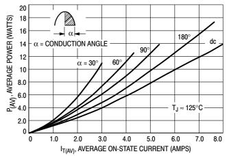
Figure 2. Maximum On-State Power Dissipation
