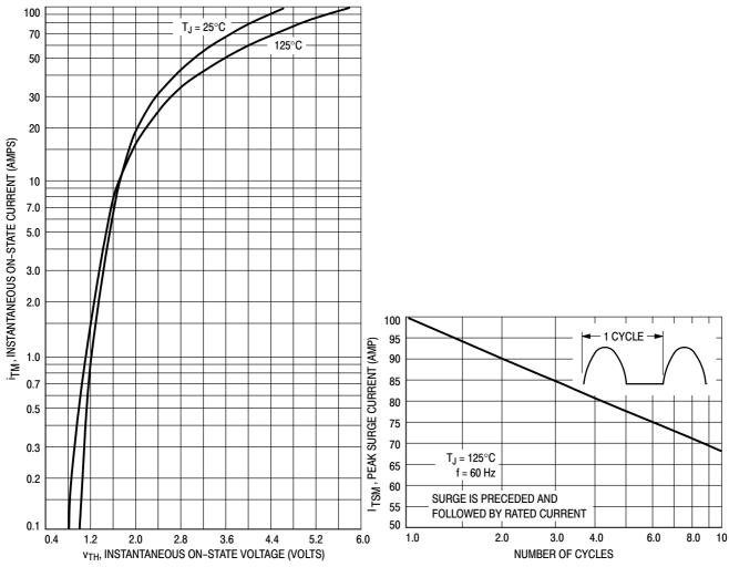
Figure 3. On-State Characteristics Figure 4. Maximum Non-Repetitive Surge Current
